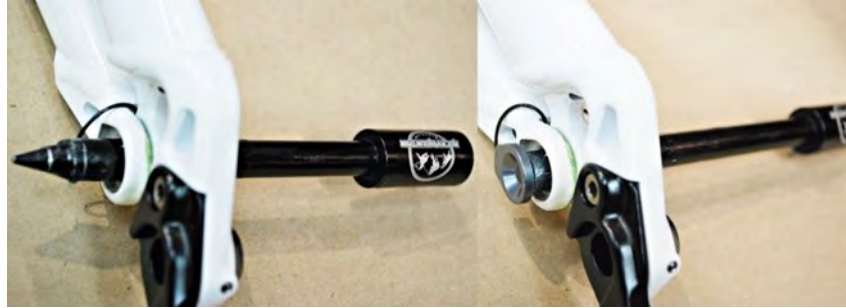
Fig 2.1.4 Drift tool used to align seat/stay chain stay pivot
