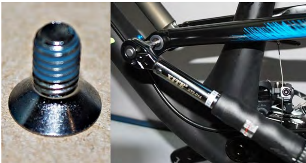
Fig. 2.3.4 Screw with Loctite and torqued to 6.7–9.0 N-m
