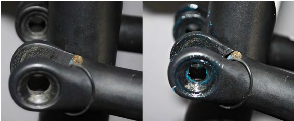
Fig. 2.7.3 O-ring positioned on outboard clevis and greased clevis
