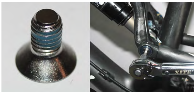
Fig. 2.7.7 Apply Loctite to the screw and torque it to 6.7-9.0 N-m
