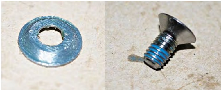
Fig. 2.1.5 Greased conical washer and Loctite coated screw
