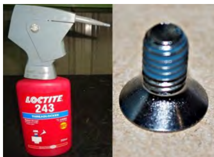
Fig. 1.6.1 Apply enough Loctite 243 to evenly coat the threads of the screws
