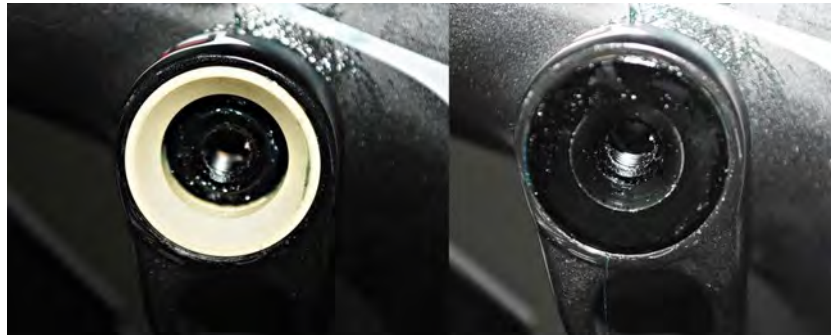
Fig. 2.8.3 Greased bushing with counter-sunk ABC washer installed
