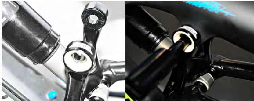
Fig. 2.5.1 Positioning the link on the top tube
