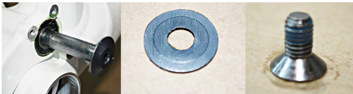
Fig. 2.2.4 Main pivot hardware
