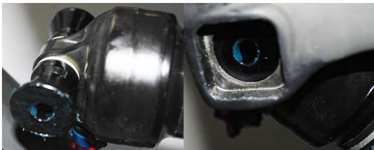
Fig. 2.6.1 positioning the front shock spacers
