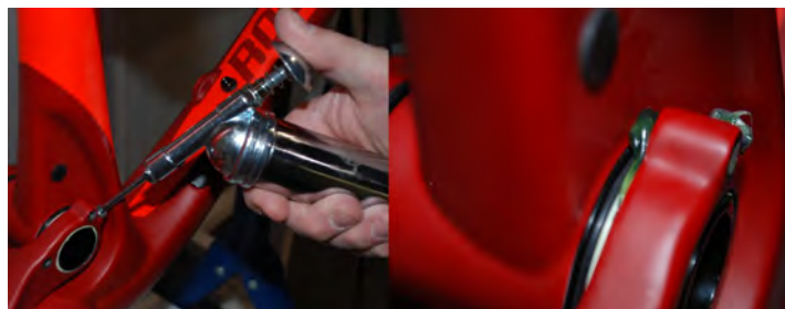
Fig. 2.10.6 Inject grease into the grease ports
