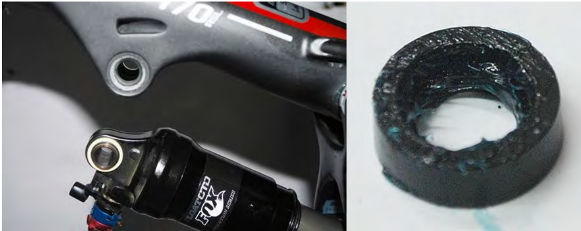
Fig. 2.9.1 Grease the forward shock spacers
