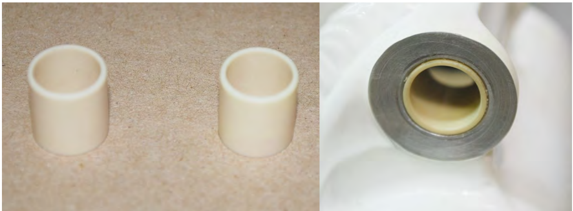
Fig. 2.2.1 Main pivot bushings before and after installation
