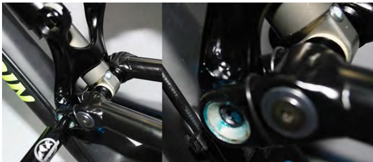
Fig. 2.4.3 Link positioned on seat stays and pivot bolt inserted
