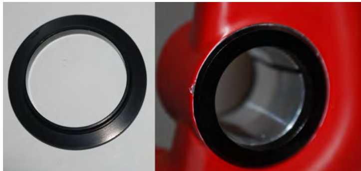
Fig. 2.10.2 Thrust washers pressed into the frame
