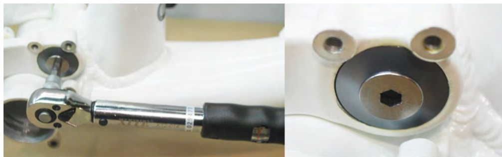
Fig. 2.2.5 Torque the main pivot bolt to 11.3 - 12.4 N-m
