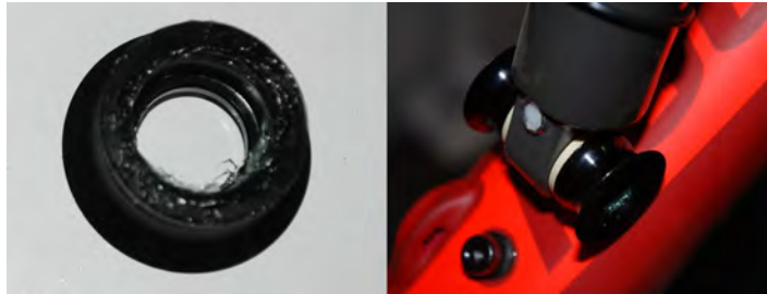
Fig. 2.11.1 Grease the shock reducers and place them on the shock
