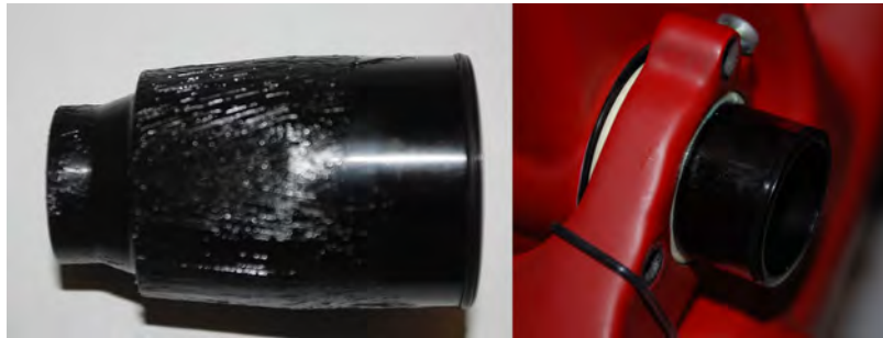
Fig. 2.10.4 Grease axle halves pressed into the chain stay
