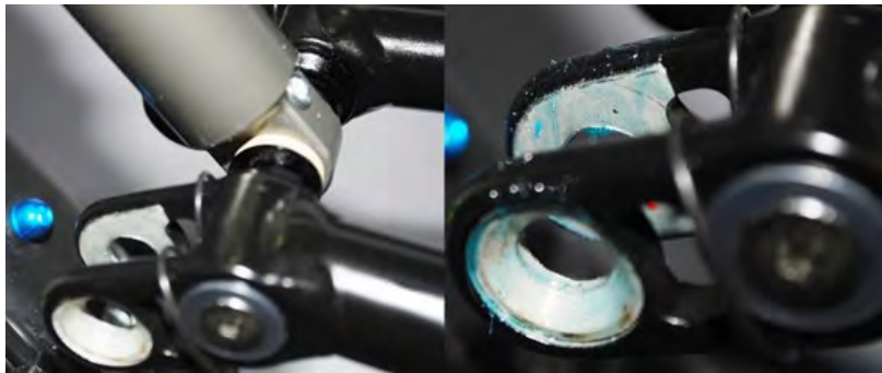
Fig. 2.4.2 O-rings positioned and greased seat stays
