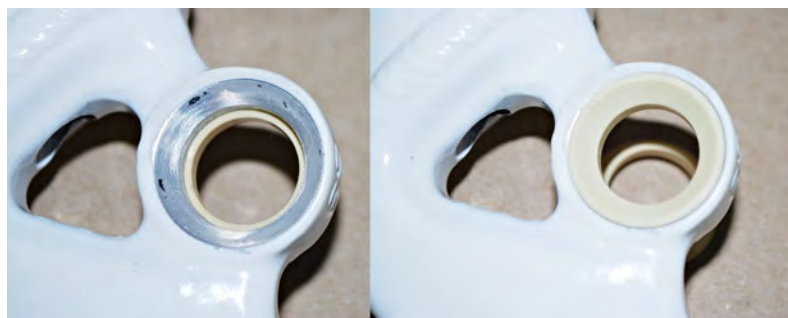
Fig. 2.1.2 Seat stay ABC surface before and after bushing installation
