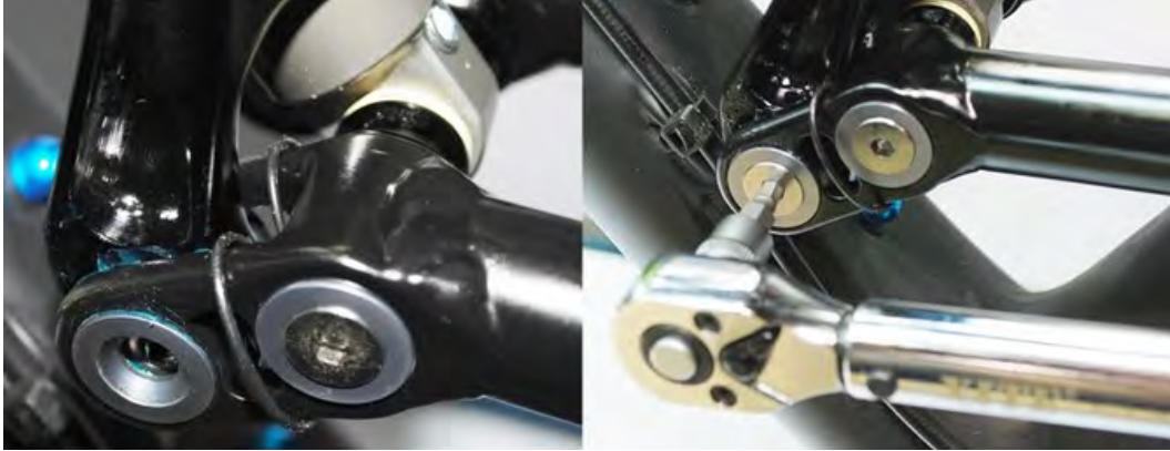
Fig. 2.4.4 Conical washer and screw being torqued to 6.7-9.0 N-m
