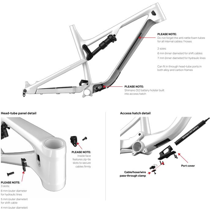
4 mm (outer diamete for electrical wire
