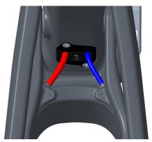
**5.** Push the cable from the rear until it comes out at the head tube port.
