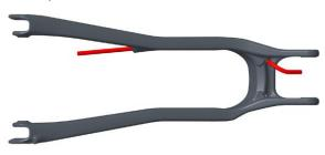
**3.** Guide the brake hose into the housing port above the bottom bracket. Make sure you insert the derailleur housing into the port labeled "Brake." The standard port is the outside one, the moto / reverse port is the middle one.
