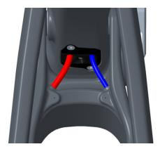
**4.** Push the brake hose from the rear until it comes out at the head tube port.
