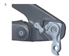
3. The UDH hanger is only compatible with the SRAM Maxle Stealth Rear Thru Axle - 12x148, 171.5mm Length, part number 00.4318.005.033
