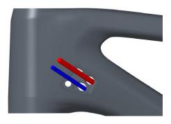
**5.** Once the hose is re-attached to the brake lever, re-install the headtube port.
