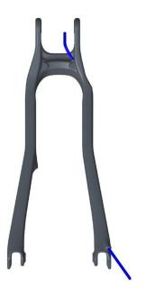
**4.** Guide the housing into the housing port above the bottom bracket. Make sure you insert the derailleur housing into the port labeled "Shift."
