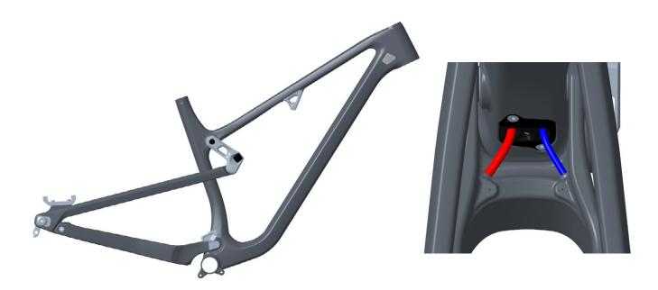
The tube-in-tube channels in the chainstay can be a tight fit, especially with the curves they have to navigate to get around the chainstay bridge. Spray soapy water or isopropyl alcohol into the opening as a lubricant to help with fitting the housing from one end to the other. Do not use grease or oil; this will leave a mess and attract dirt.
