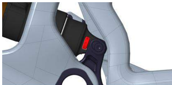
Chip in 29 position
